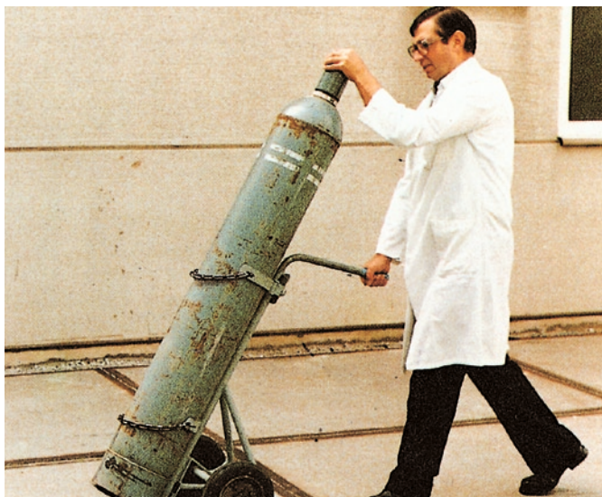
Picture 14: Pressurized gas cylinders must be secured by chaining up against tilting both during transport on the carts designed for this purpose and on-site.
